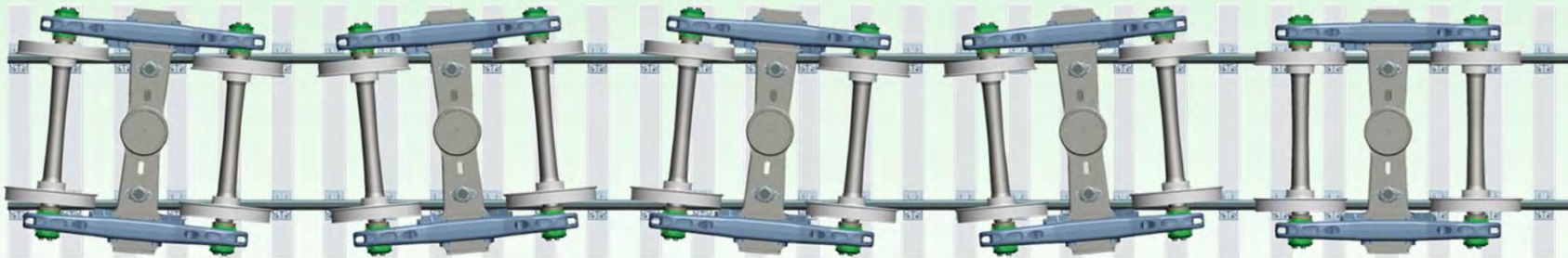
Truck Hunting Truck Warp, Truck Rotation, Wheelset Movement 40+ mph
